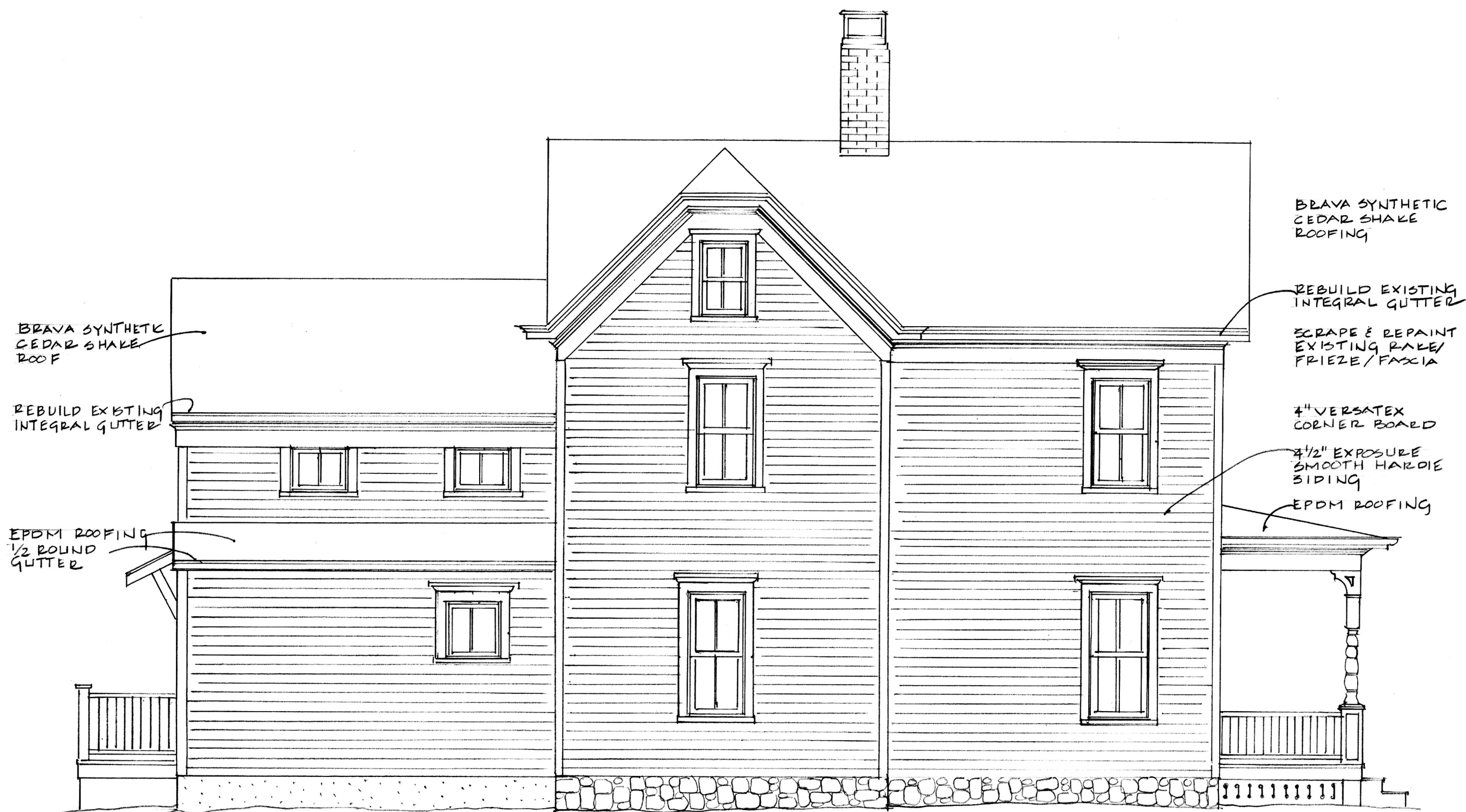
SIDE / NORTH ELEVATION 1/4" = 1'-0"
